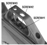
SCREW#1 is for trigger pull force adjustment. For less trigger pull force prior to discharge, rotate SCREW#1 clockwise; and vice versa. SCREW#2 is for trigger travel adjustment.
